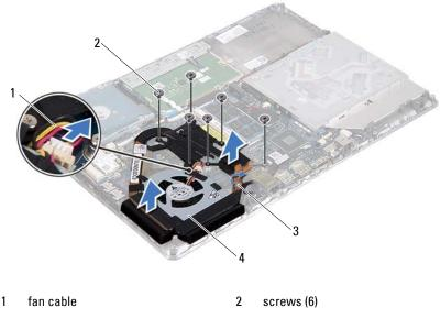
3 display cable tape 4 heat sink and fan
