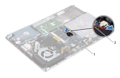
1 coin-cell-battery 2 coin-cell battery cable
